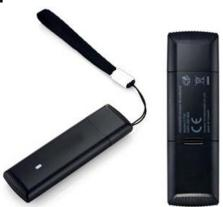
The E-Lins EL-6300d HSDPA Data Card Modem is a complete 3.5G/3.75G enabled wireless USB data modem designed to offer high-speed wireless connectivity for Windows notebook and desktop computers on HSDPA/HSUPA networks. It is easy to use USB connector and the ability to roam globally on tri-band UMTS and quad-band GSM/ EDGE networks. It enables connection to internet download speed up to 7.2Mbps.
