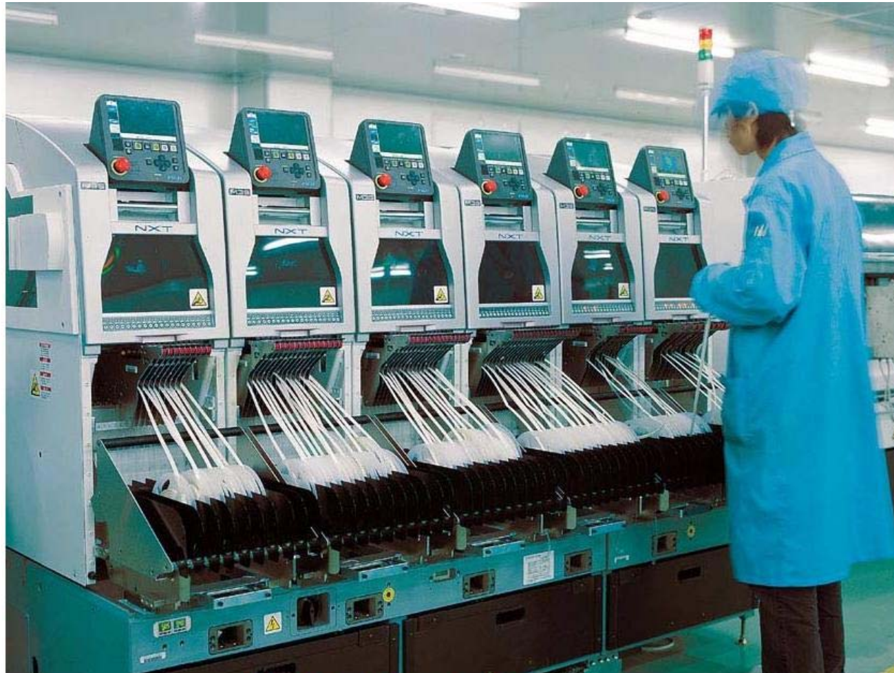
Modular Mounter Room
